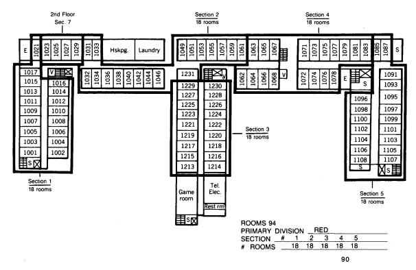
**Figure 2-8** House Breakout Plan of the model hotel; first floor. S, storage; V, vending; E, electrical switch room; X, elevator; GL, guest laundry.
